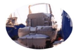
Even a brief cold spell that lasts only a night or two can do considerable damage. In temperate states, boat owners must winterize engines and freshwater systems, especially when boats are stored ashore. In deep freeze states, boats stored ashore must be winterized earlier than boats stored in the water.
