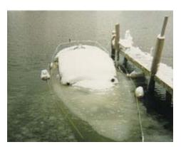
A plastic thru-hull that was an inch or two above the waterline cracked and the weight of the snow lowered the damaged fitting to just below the surface. The boat gradually filled with water and sank.
